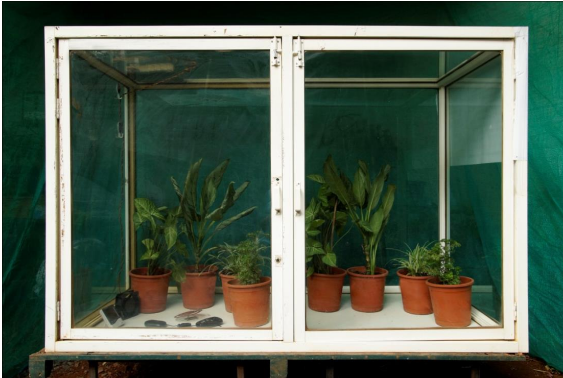
Photo 1 : Glass chamber for treatment having two compartments, Treatment and control
